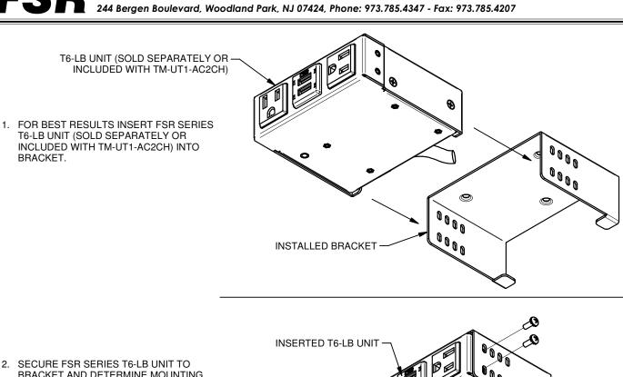
2. SECURE FSR SERIES T6-LB UNIT TO BRACKET AND DETERMINE MOUNTING LOCATION ON TABLE UNDERSIDE.
