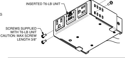
3. REMOVE T6-LB UNIT FROM BRACKET. USE BRACKET AS TEMPLATE FOR PILOT HOLES AND SECURE BRACKET TO TABLE WITH SUPPLIED MOUNTING SCREWS. REINSTALL T6-LB UNIT AND MAKE ELECTRICAL CONNECTIONS AS REQUIRED.
